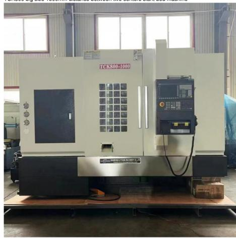
**High-Precision Machining**: With a positioning accuracy and repeat accuracy of 0.01 mm, it guarantees precise machining for components requiring high accuracy.
