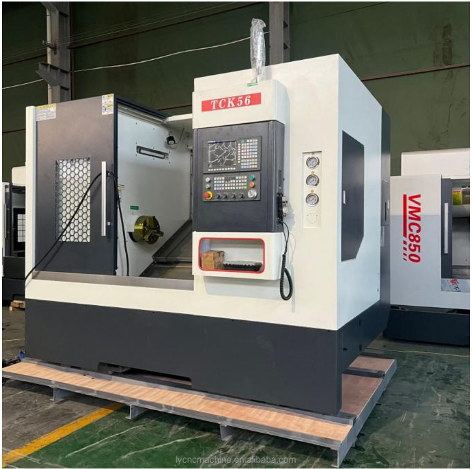
TCK slant bed cast iron body
