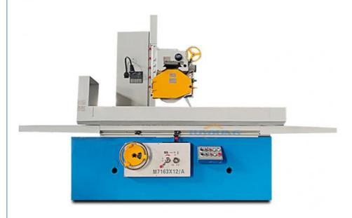
The M7163x1250 surface grinding machine is an efficient grinding machine tool with several notable features, suitable for various machining needs. Here are its main characteristics:
