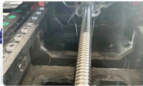
TAIWAN HIWIN LINAER GUIDEWAY & BALL SCREW
