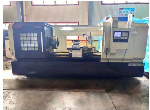
The distance between two centers: 2000mm The cnc control system: standard---- GSK928 control system Optional: Siemens/Fanuc/Syntec and etc.
